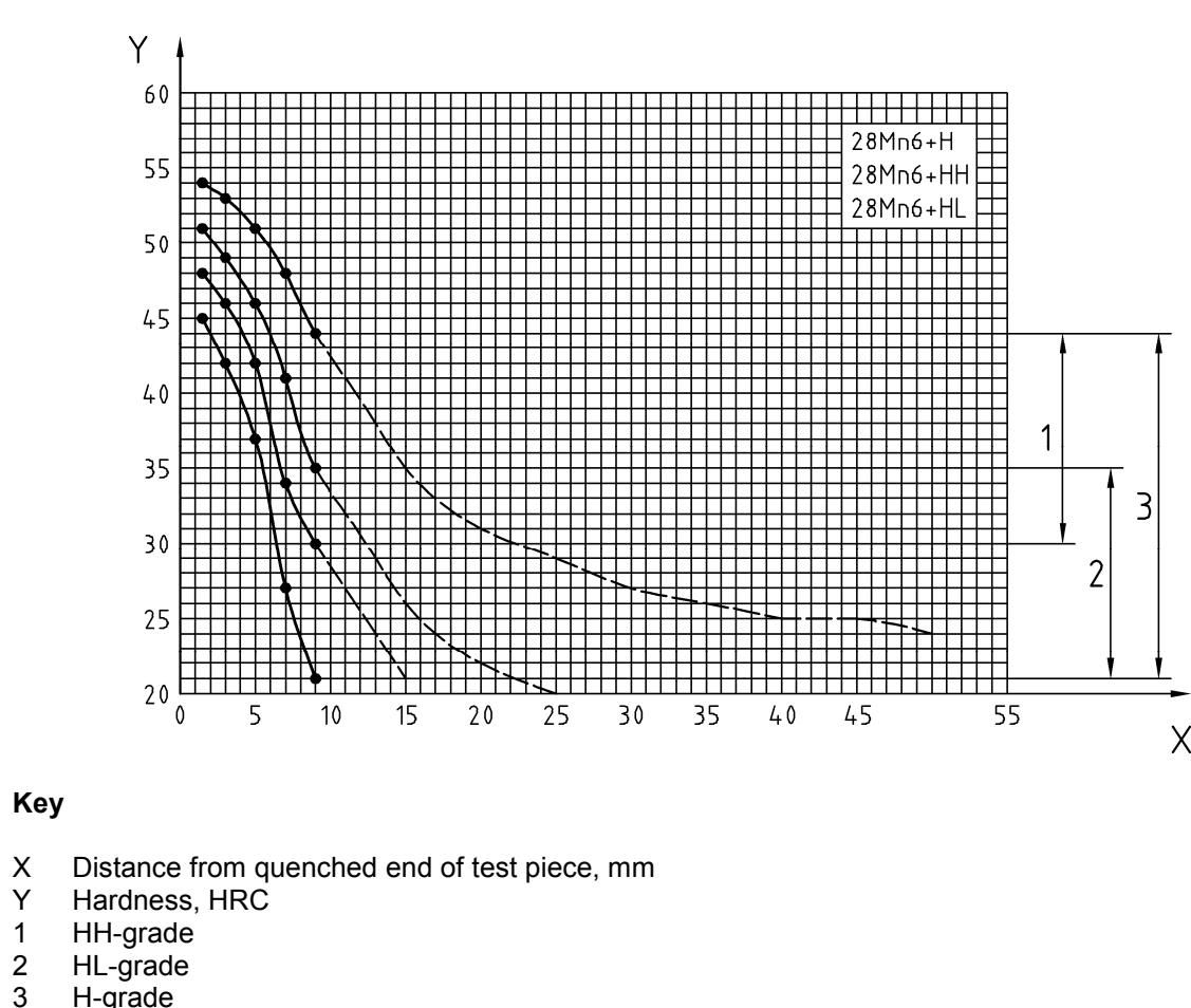
**Figure 1g — Scatter bands for the Rockwell-C hardness in the end quench hardenability test**
